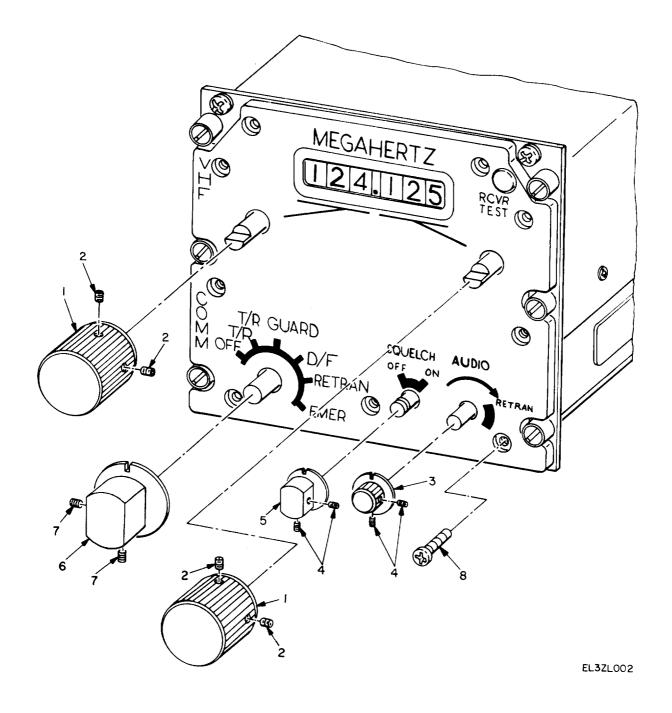
Figure 2. Panel Assembly, Radio Set AN/ARC-115A(V)l.
